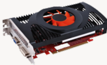
Graphic card with ventilator for cooling.
